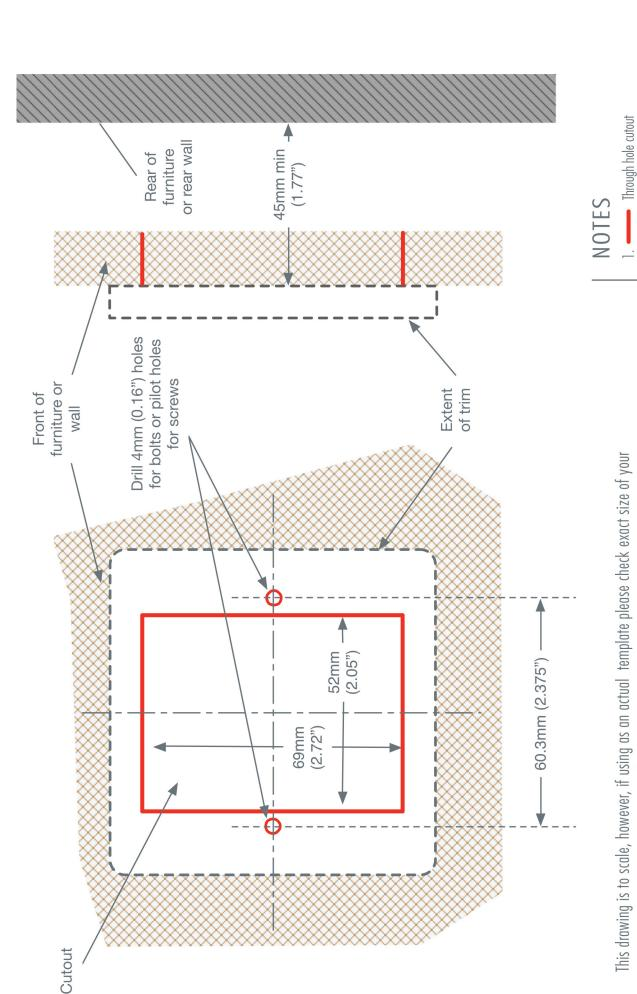
This drawing is to scale, however, if using as an actual template please check exact size of your print out as output on printers can shift drawing scale.
