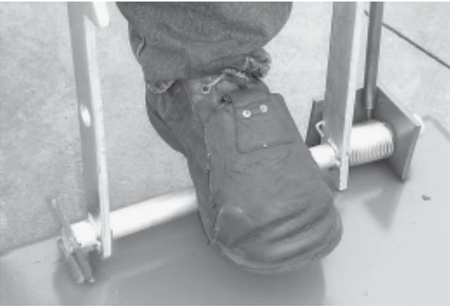
The release assembly pin will line back up with the hole in the end bracket.
