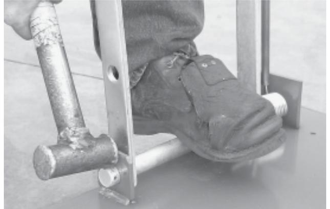
Use the hammer to push the end of the bracket back to an upright / straight position.
