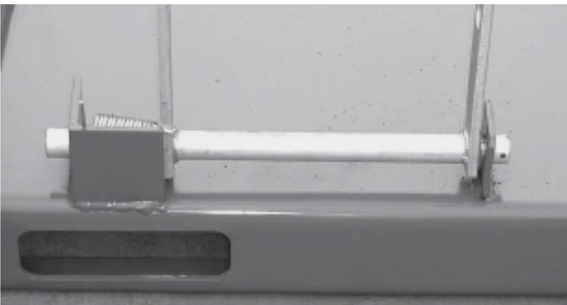
H-Style installed spring and release lever assembly.
