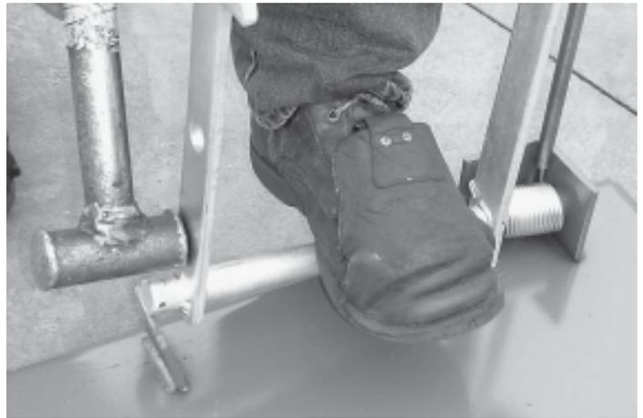
Use a hammer to push the release lever assembly towards the angled bracket while pushing down on the locking finger.
