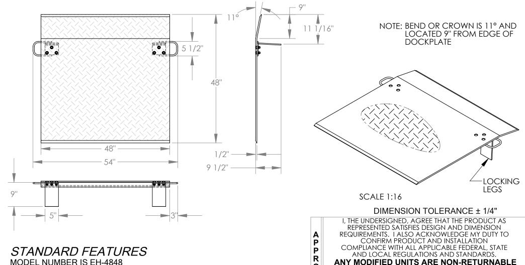
MODEL NUMBER IS EH-4848 CAPACITY IS 3,800 LBS. OVERALL WIDTH IS 54" DECK WIDTH IS 48" OVERALL LENGTH IS 48" OVERALL HEIGHT IS 9 1/2" THICKNESS IS 1/2" HANDLES ARE 5 1/2" x 3" LOCKING LEGS ARE 5" x 9"
