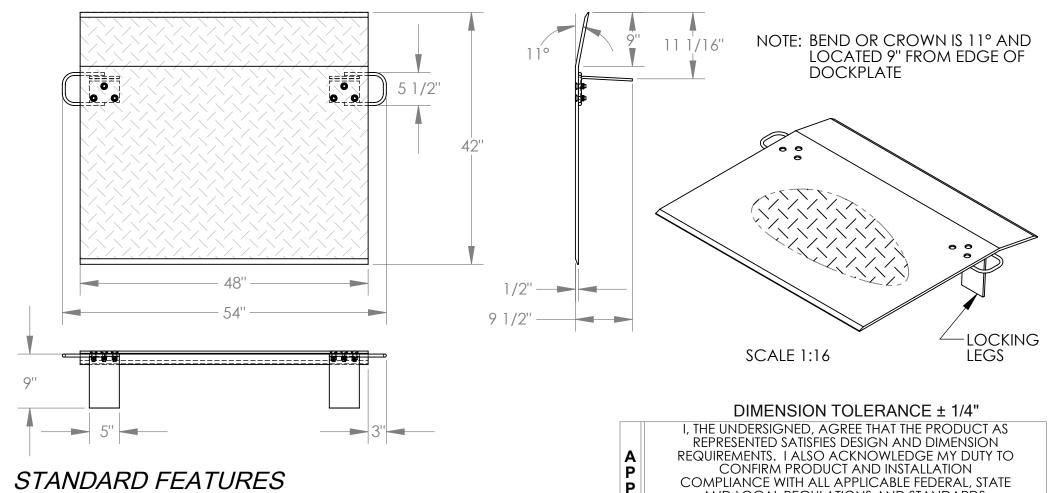
**MODEL NUMBER IS EH-4842** CAPACITY IS 4,300 LBS **OVERALL WIDTH IS 54" DECK WIDTH IS 48" OVERALL LENGTH IS 42" OVERALL HEIGHT IS 9 1/2"** THICKNESS IS 1/2" HANDLES ARE 5 1/2" x 3" LOCKING LEGS ARE 5" x 9"
