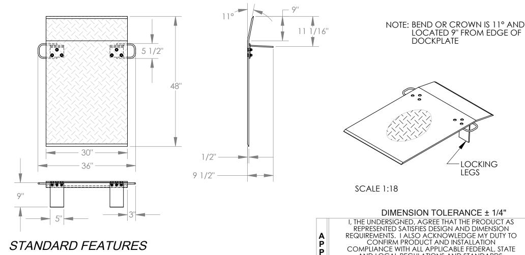
MODEL NUMBER IS EH-3048 CAPACITY IS 2,600 LBS. **OVERALL WIDTH IS 36" DECK WIDTH IS 30" OVERALL LENGTH IS 48"** THICKNESS IS 1/2" **OVERALL HEIGHT IS 9 1/2"** HANDLES ARE 5 1/2" x 3" LOCKING LEGS ARE 5" x 9"
